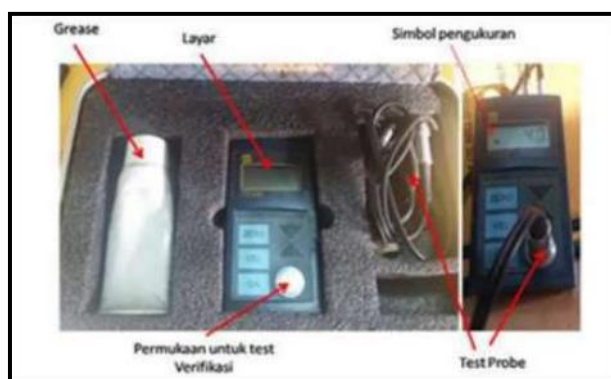
Gambar 1. Smart Sensor Ultrasonic Thickness Gauge TT 130
